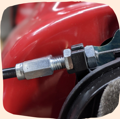
Figure 6: Jam nuts in the "forward" position
