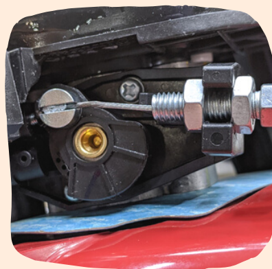
Figure 5: Throttle "fully closed"; throttle body rests on the set screw
