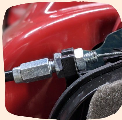
Figure 7: Jam nuts in the "backwards" position
