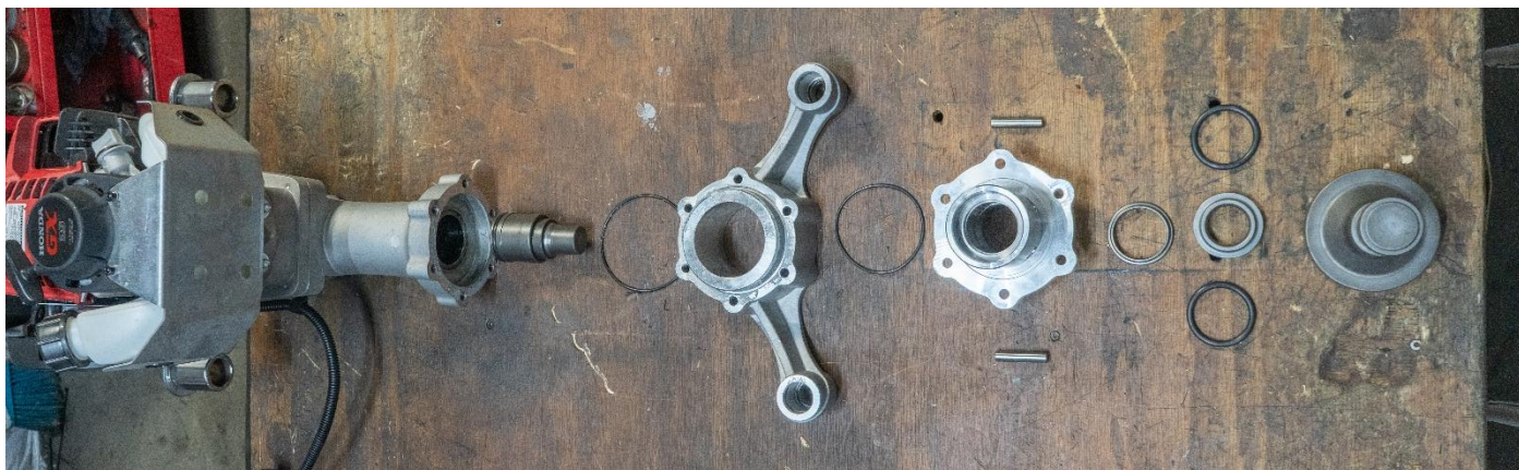
Figure 8: View when lower driver body is removed
