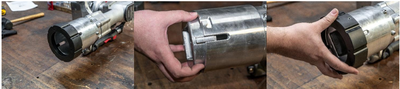
Figure 4: Installing the guide collar in a PGD4000X-DOT
