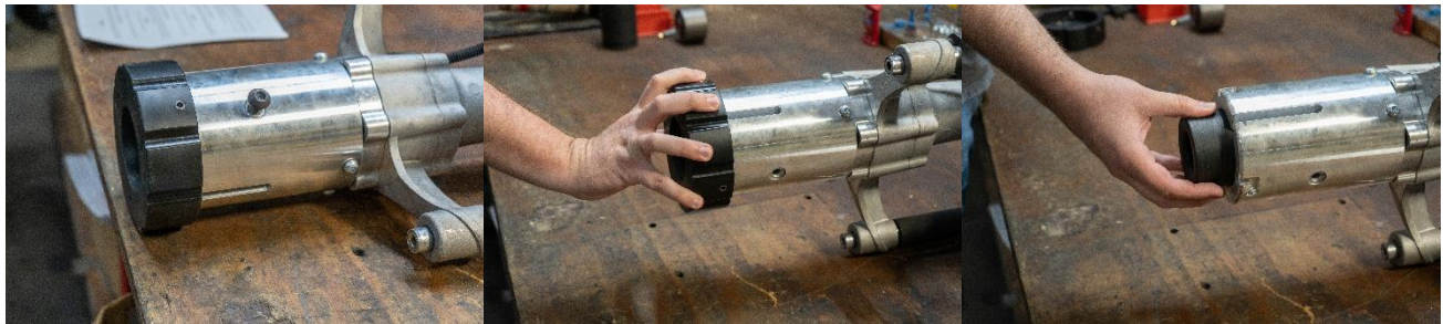
Figure 2: Installing the adapter sleeve on a PGD4000X-PFR
