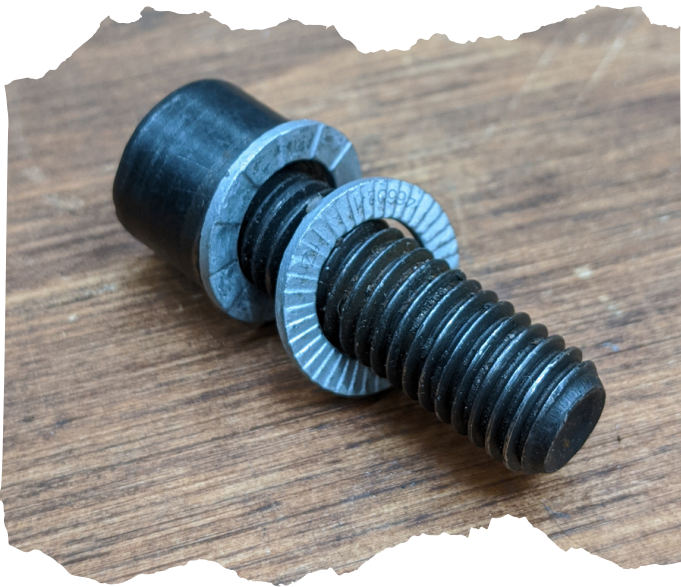
Figure 1: Proper orientation of lock washers on M10x40mm cap screw
